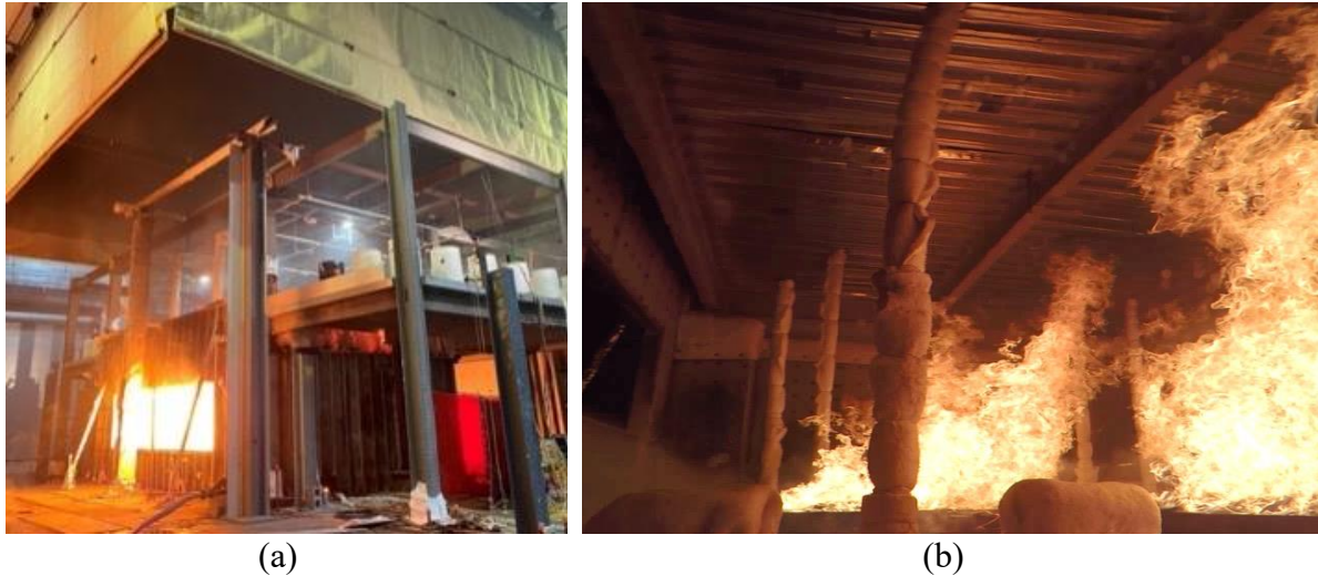
Fig. 1. (a) Compartment fire test in the south middle bay of the two-story building under 20 MW exhaust hood; (b) Composite floor soffit exposed to natural gas fueled compartment fire.
