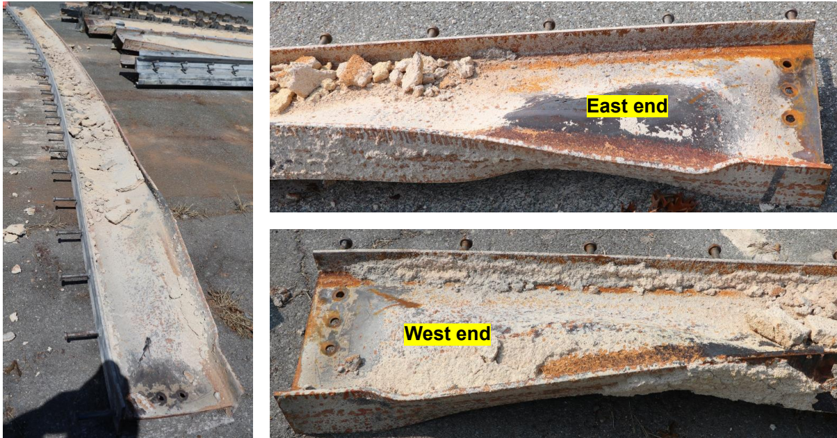
Fig. 73. Post-test photographs: South edge beam.
