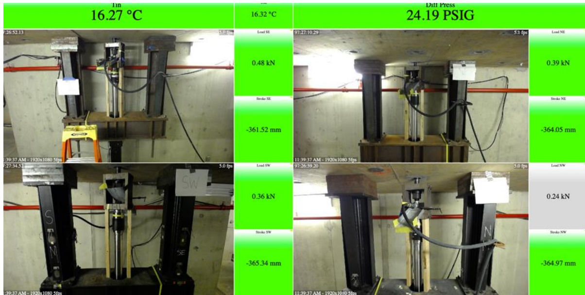
Fig. 39. Screenshot of the test video to monitor hydraulic actuators at the basement of the NFRL strong floor (prior to fire testing).
