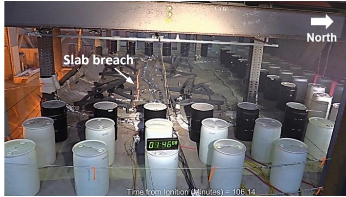
Fig. 2. Still image showing top of the Test #1 composite floor developing slab breach at 106 min after burner ignition.
