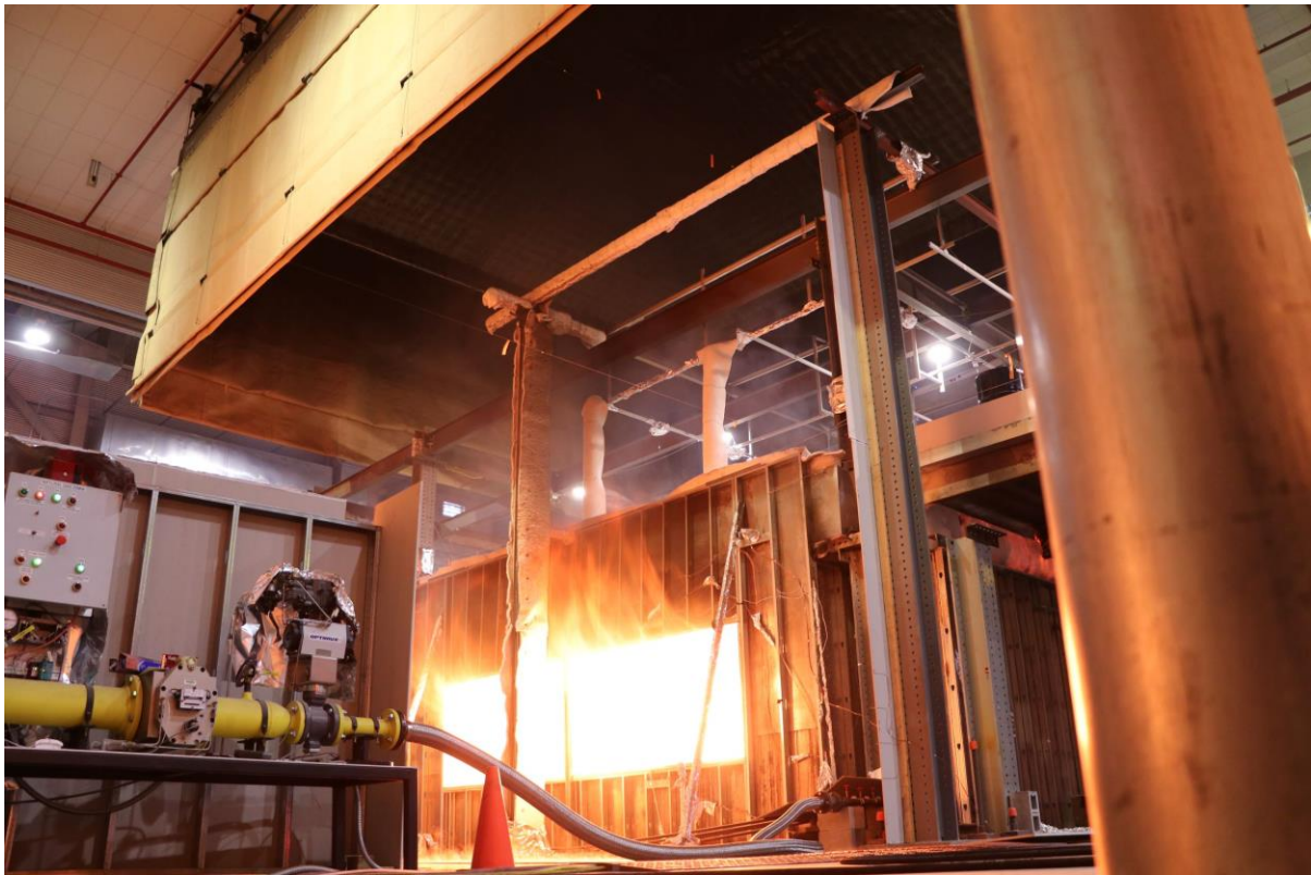
Fig. 18. Front view of the main vent opening of the fire test compartment during Test #2.
